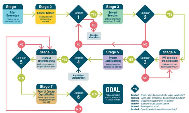
Fig. 1 Workflow for seeded continuous crystallisation.
