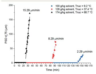
Fig. 7 Example growth rates from Crystalline PSD.
