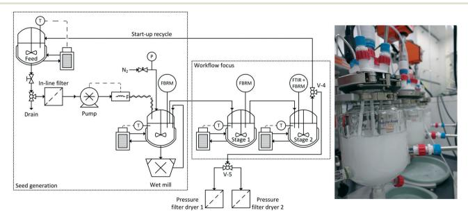
Fig. 11 Process and instrumentation diagram of configuration for stage 7.
