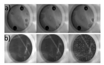
Fig. 5 Sequential fouling images for a) borosilicate (0, 205 and 602 min) and b) Hastelloy® C276 (0, 107 and 653 min) at S = 2.00.
