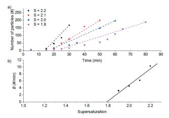
Fig. 4 a) Particle count, N, in arbitrary units against time for seeded secondary nucleation experiments at different supersaturation ratios. b) Observed secondary nucleation rate, B, in arbitrary units as a function of the supersaturation in the seeded experiments.
