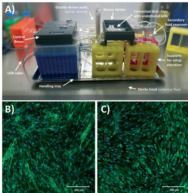
**Fig. 8** A) Closed-loop gravity-driven setup used for cell-culture experiment. B) Confocal microscopy of endothelial cells cultured under static conditions as control. C) Confocal microscopy of endothelial cells cultured under 4 cm of closed-loop gravity-driven flow. Both cultures present with no observable differences, which suggests appropriate biocompatibility of the system.
