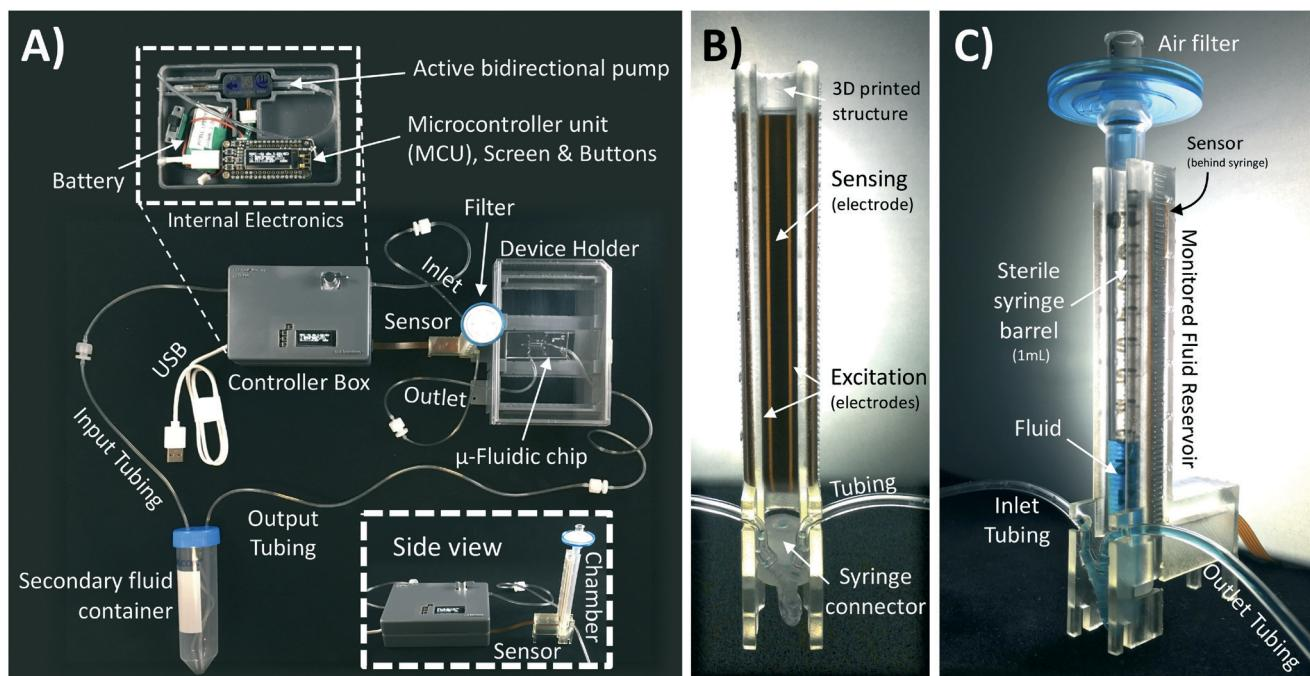
**Fig. 2** A) Fabricated testing setup used to perform the validation experiments of height-based closed-loop control of open-well microfluidic systems. B) Detail of embedded non-contact capacitive fluid-level sensor with custom-designed electrodes. C) Assembled gravity driven reservoir with embedded capacitive sensing and a single upper air filter (0.22  $\mu\text{m}$  pore size) for sterile use in cell culture applications.
