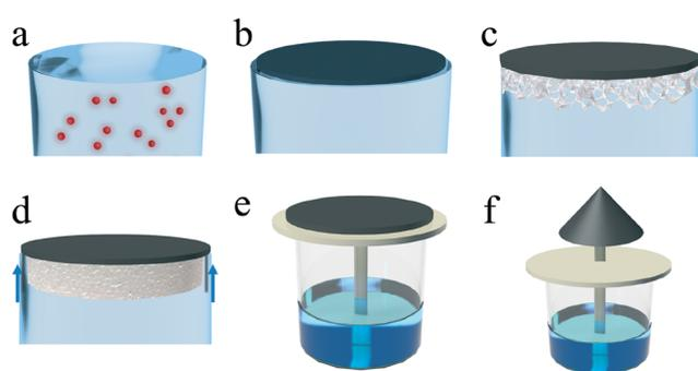
**Fig. 3** Evolution of photothermal structures for solar evaporation. (a) Dispersed nanoparticles for bulk water heating; self-floating 2D photothermal materials (b) without a heat barrier, (c) with a macroporous heat barrier, and (d) with a nonporous heat barrier and 2D water channels; (e) 2D and (f) 3D photothermal materials with 1D water channel.
