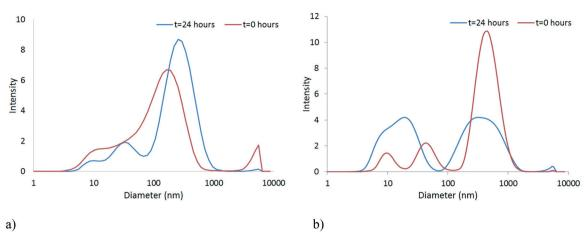
Fig. 3 Size distribution graphs at time 0 and after 24 hours for a) CeO<sub>2</sub> b) ZnO in the unconditioned HH Combo medium.
