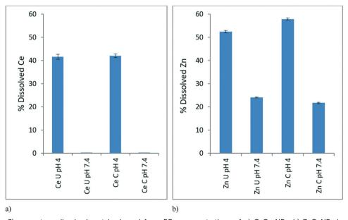
Fig. 4 Average (n = 3) percentage dissolved metal released from EC<sub>10</sub> concentrations of a) CeO<sub>2</sub> NPs, b) ZnO NPs in conditioned (C) and unconditioned (U) medium at pH 4 and pH 7.4, as determined by ICP-OES following centrifugal separation of the ionic fraction. The dissolution of CeO<sub>2</sub> NPs at pH 7.4 was minimal (<0.05%).
