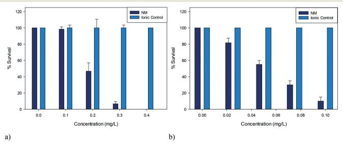
Fig. 2 Percentage survival of D. magna juveniles exposed to a) 5 nm PVP capped  $CeO_2$  NPs b) 5 nm PVP capped ZnO NPs and their corresponding ionic controls (n = 3).
