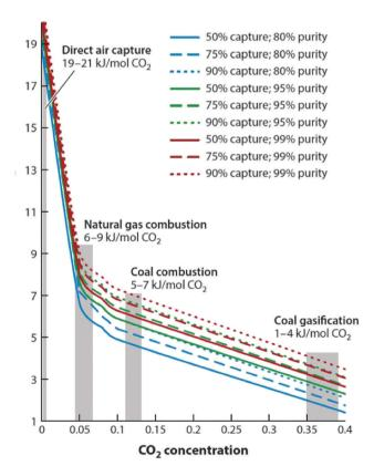
Fig. 27 Minimum work required for CO<sub>2</sub> capture based upon initial CO<sub>2</sub> concentration, capture rate, and final CO<sub>2</sub> purity. 308
