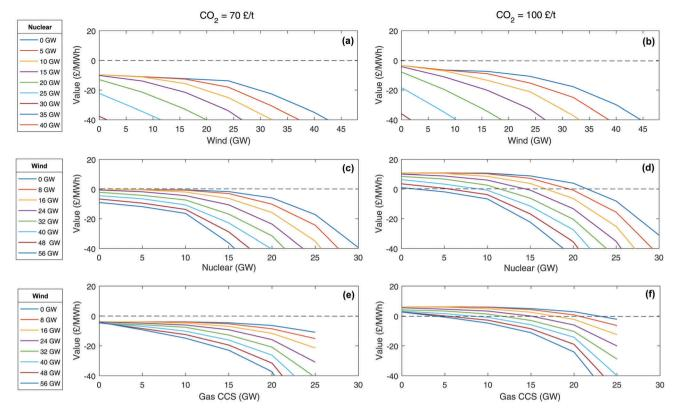
Value of technology addition (VOTA) or system value of building of wind, nuclear and gas CCS technology
