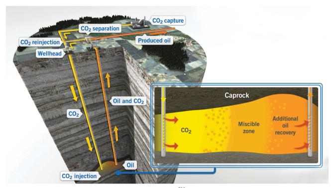
Fig. 19 Schematic diagram of CO<sub>2</sub>-EOR process. Source: Global CCS Institute. 964
