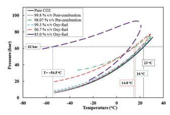
Fig. 17 Boundaries of VLE region in pressure—temperature phase diagram for pure CO $_2$ , pre-combustion, post-combustion and oxy-fuel streams (85 and 96.7% v/v CO $_2$ ) calculated using PR EoS.  $^{808}$
