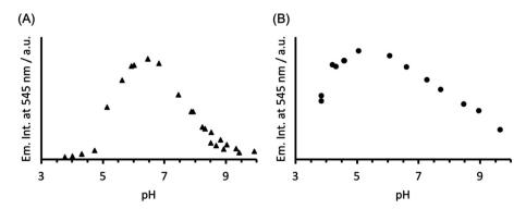
Fig. 6 Plot of the change in emission intensity at 545 nm as a function of pH, for a solution containing 30  $\mu$ M (A) CS1-1 and (B) MB1-2 monomer in the presence of 10  $\mu$ M TbCl<sub>3</sub>.  $\lambda_{exc}$  = 280 nm.
