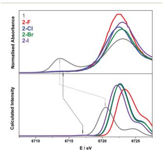
Fig. 7 Comparison of the experimental (top) and calculated (bottom) Sm L<sub>3</sub>-edge spectra of 1 (grey), 2-F (red), 2-Cl (blue), 2-Br (green) and 2-I (violet) obtained from the ZORA-PBE0 TD-DFT calculations. The calculated spectra are shifted +78.6 eV with the intensity in arbitrary units. The grey dashed line links the experimental and calculated Sm(II) white-line peaks; the black dashed line links the experimental and calculated Sm(III)-X pre-edge peaks.
