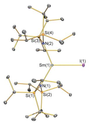
Fig. 4 Molecular structure of  $[Sm(N^{\dagger\dagger})_2(I)]$  (2-I) with selective atom labelling. Displacement ellipsoids set at a 30% probability level and hydrogen atoms are omitted for clarity. Selected bond lengths [Å]: Sm(1)-I(1) 3.0199(7), Sm(1)-N(1) 2.323(3), and Sm(1)-N(2) 2.289(3). Selected bond angles [°]: N(1)-Sm(1)-N(2) 128.07(10), N(1)-Sm(1)-I(1) 119.75(7), and N(2)-Sm(1)-I(1) 112.16(7).
