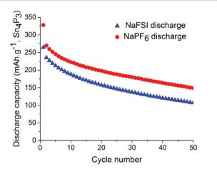
Fig. 4 Discharge capacity for symmetrical-cells with NaPF<sub>6</sub> salt (red) and NaFSI salt (blue) over 50 galvanostatic cycles. Electrodes were cycled between -1.25 V and 1.25 V in pouch cells.
