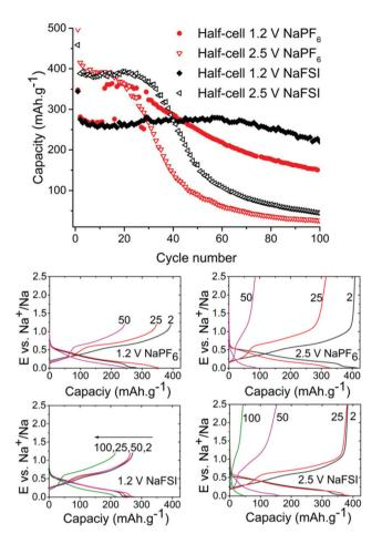
Fig. 2 Discharge capacity from galvanostatic cycling of tin phosphide at 50 mA g<sup>-1</sup> in half cells with NaFSI (black) & NaPF<sub>6</sub> (red) with upper cut-off potential set to 1.2 V and 2.5 V (top). Voltage profiles for same cells at selected cycles (bottom).
