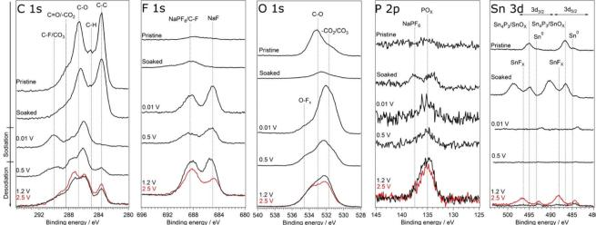
Fig. 6 HAXPES spectra of  $Sn_4P_3$  electrodes from cells with the NaPF<sub>6</sub> based electrolyte. The spectra were measured using photon energy of 2005 eV. The samples charged to 2.5 V is shown in red.
