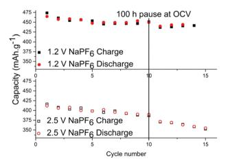
Fig. 3 Discharge and charge capacities in tin-phosphide half-cells using NaPF<sub>6</sub> before and after 100 h pause/relaxation. Top figure shows the results for the cell with 1.2 V high cut-off potential, and the bottom figure displays for the cell with 2.5 V high cut-off potential.
