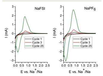
Fig. 1 Cyclic voltammogram of Sn<sub>4</sub>P<sub>3</sub> vs. sodium metal using electrolytes of 1 M NaFSI (left) or NaPF<sub>6</sub> (right) dissolved in EC: DEC (1:1) and 10 vol% FEC additive. Scan was performed between 0.01 V-2.5 V at 1 mV s<sup>-1</sup> scan rate.
