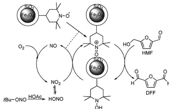
Fig. 42 Proposed reaction pathway for the aerobic oxidation of 5-hydroxymethylfurfural (HMF) into 2,5-diformylfuran (DFF) using a Fe<sub>3</sub>O<sub>4</sub>@SiO<sub>2</sub>-TEMPO catalyst. Reproduced with permission from ref. 364. Copyright (2014) John Wiley and Sons.
