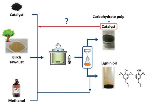
Fig. 38 A schematic representation for the catalytic reductive fractionation of lignocellulose sawdust using Ru/C catalyst in methanol under H<sub>2</sub> pressure.
