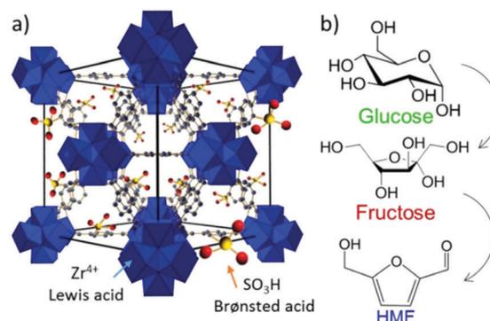
Fig. 26 (a) Schematic representation of an acidic UiO-66 framework. (b) Conversion of glucose to HMF *via* fructose isomerisation. Reproduced with permission from ref. 246. Copyright (2018) John Wiley and Sons.
