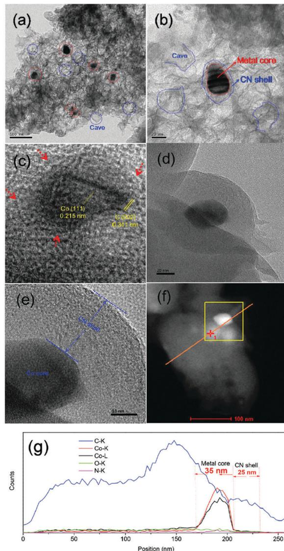
Fig. 20 TEM images (a–e), STEM image (f) and line scanning EDS elemental analysis (g) of  $\text{Co}@\text{NC}$ -700 catalyst. Reproduced with permission from ref. 72. Copyright (2017) Royal Society of Chemistry.
