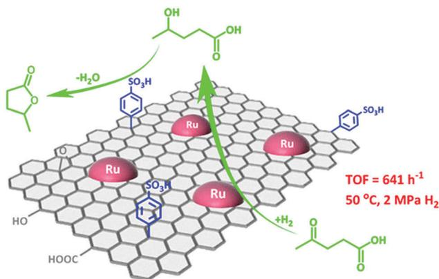
Fig. 5 Graphene-based metal/acid bi-functional catalyst for one-pot conversion of levulinic acid to  $\gamma$ -valerolactone. Reproduced with permission from ref. 79. Copyright (2017) American Chemical Society.
