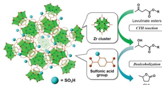
Fig. 21 SO<sub>3</sub>H-Functionalised UiO-66 MOF for catalytic transfer hydrogenation (CTH) of levulinate esters to  $\gamma$ -valerolactone. Note: Zr and O atoms are shown in green and brown, respectively. Reproduced with permission from ref. 222. Copyright (2017) American Chemical Society.
