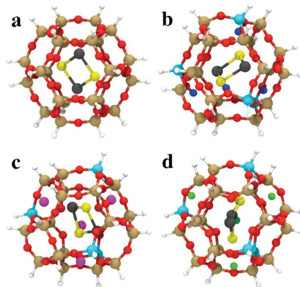
**Fig. 5** The most stable  $(\text{PbS})_2$  adsorption configurations in (a) SiSOD, (b) HSOD, (c) LiSOD and (d) NaSOD cages, described by an H-terminated cluster model at the PBE0/TZVP level of DFT. O is red, Si is brown, Al is cyan, Li is magenta, Na is green, Pb is black, S is yellow, terminating-H is white, charge-compensating  $\text{H}^+$  is blue. Reprinted with permission from ref. 147. Copyright 2016, American Chemical Society.
