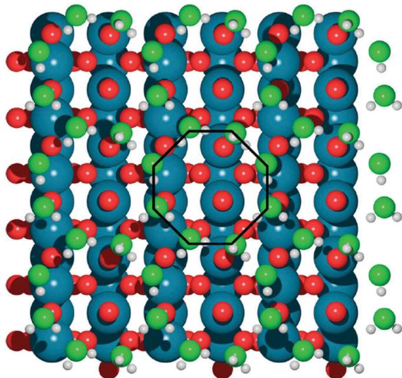
Fig. 2 The optimal, octahedral structure of a water bilayer upon IrO<sub>2</sub>, determined with DFT minima-hopping. Water oxygen atoms are light green, surface oxygen atoms are red, iridium is blue and hydrogen is white. Reprinted with permission from ref. 18. Copyright 2017 American Chemical Society.
