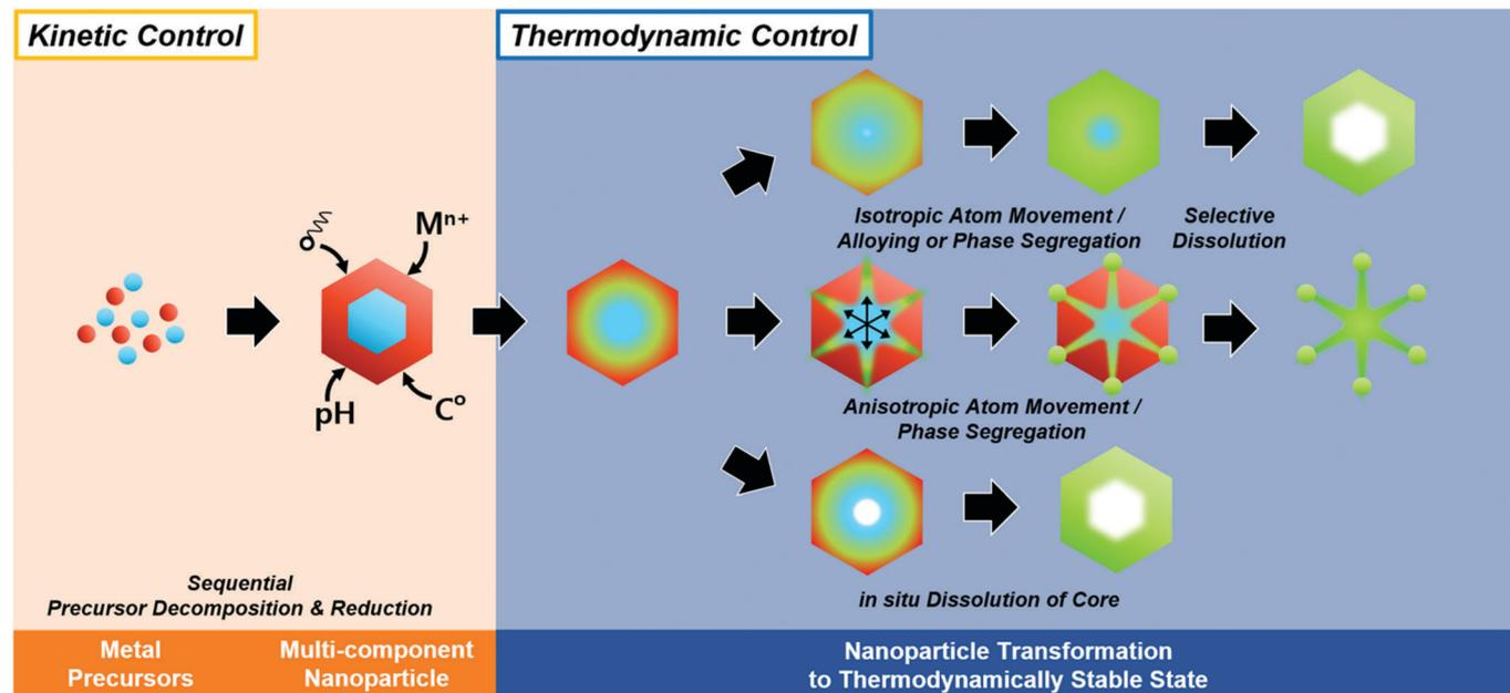
Fig. 6 Schematic illustration of *in situ* formed template-mediated synthetic approach toward hollow nanostructures with kinetic and thermodynamic control.
