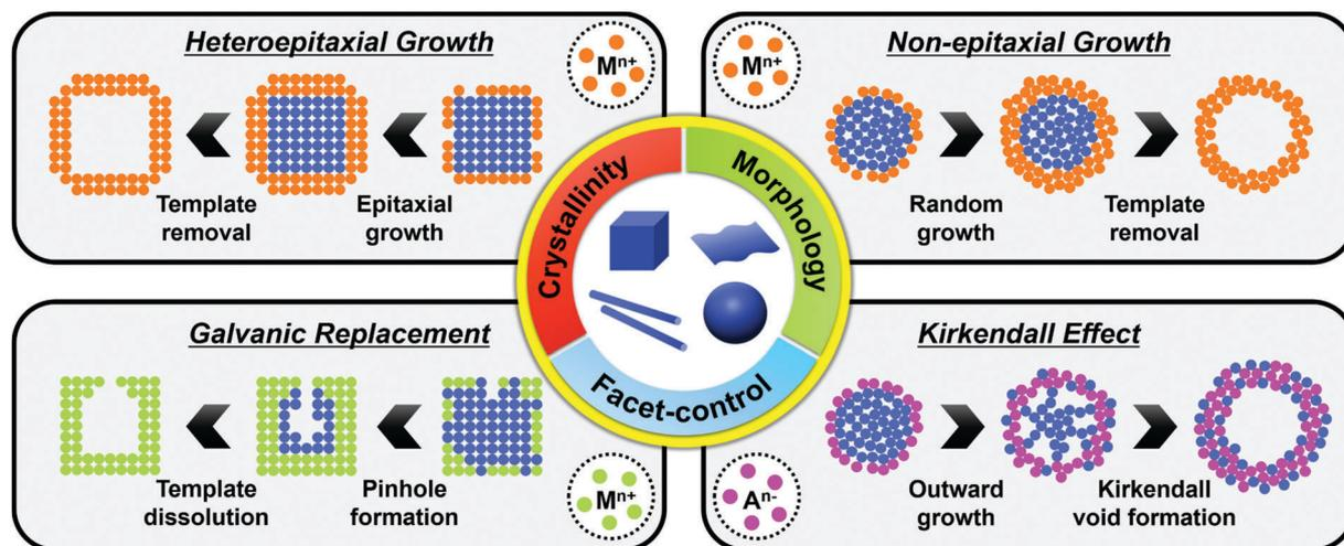
**Scheme 1** Representative schematic diagram of synthetic methodologies to hollow nanostructures by using various pre-synthesized templates. The physical and chemical properties of resulting hollow nanostructures are heavily dependent on various factors, such as crystallinity, morphology, dimensionality, and exposed facets, of the engaged templates.
