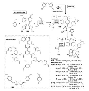
Fig. 21 Preparation of monolithic polymers by polymerization of vinylic
