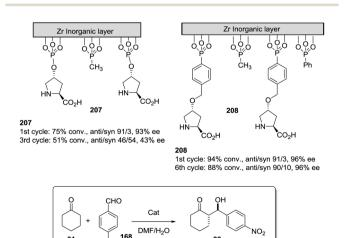
Fig. 50 Proline supported on zirconium through phosphate or phosphonate bonds and studied as an organocatalyst for aldol reactions.
