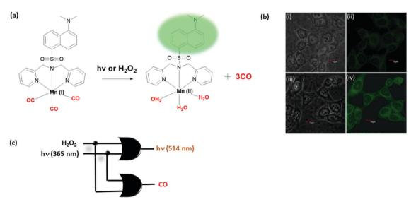
Fig. 16 Two OR logic gates generated through light and hydrogen peroxide mediated CO release. (a) Chemical structure of a CO-releasing Mn complex. (b) Confocal microscopy images of HCT116 colon cancer cells: (i and iii) bright-field images, (ii) image without illumination, and (iv) image illuminated with 405 nm LED light. (c) Logic gate diagram. Reproduced with small alterations from ref. 31 with permission from Royal Society of Chemistry, copyright 2017.
