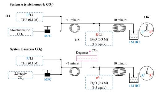
Fig. 17 Organolithium mediated continuous flow synthesis of ketones.
