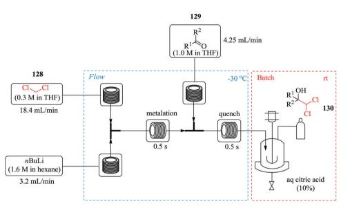
Fig. 20 In situ generation and electrophilic quench of dichloromethyllithium in continuous flow reactors.
