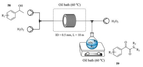
Fig. 5 Continuous flow set up for the synthesis of  $\alpha$ -amino ketones.
