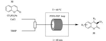
Continuous flow trifluoromethylation using Langlois reagent.
