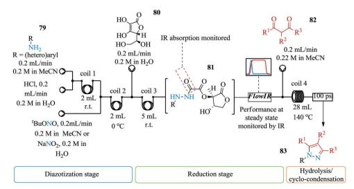
Fig. 9 Multi-step continuous flow synthesis of pyrazoles via a metal free amine-redox process.
