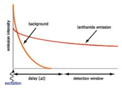
Fig. 2 Time-resolved luminescence measurements. The sample is irradiated with a pulse at the excitation wavelength, and the emission intensity is recorded after a delay time ( $\Delta t$ ) for a defined period (detection window).
