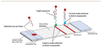
Fig. 1 Schematic depicting the lateral flow assay.
