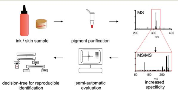
Scheme 1 Highly specific identification of water-insoluble organic pigments is facilitated by automated matrix-assisted laser desorption/ionization tandem mass spectrometry. Semi-automated evaluation following a decision-tree allows for reproducible identification in complex matrices for market surveys and research of tattoo-derived side effects.
