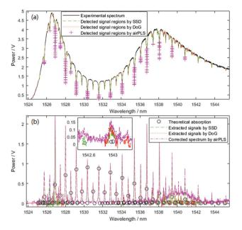
Fig. 8 Experimental data of C<sub>2</sub>H<sub>2</sub> absorption spectrum: (a) signal region detection and (b) signal extraction.
