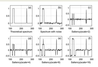
Noise influence. The maximum saliency of the square signal is not at the centre of the signal and is not obtained when the scale equals half-breadth.
