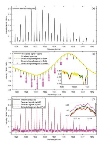
Fig. 6 Simulated data of C<sub>2</sub>H<sub>2</sub> absorption spectrum: (a) theoretical spectrum, (b) signal region detection and (c) signal extraction.
