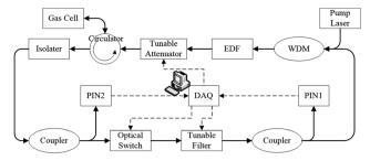
Fig. 4 Schematic of the C<sub>2</sub>H<sub>2</sub> experiment system.
