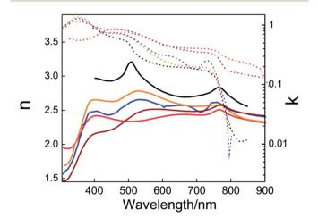
Fig. 1 Real part of the refractive index (n, continuous line) and extinction coefficients (k, dashed lines) of MAPI perovskite layers prepared employing different techniques. Data were adapted from the following references: black;<sup>42</sup> orange;<sup>43</sup> blue;<sup>44</sup> brown;<sup>45</sup> red.<sup>46</sup>
