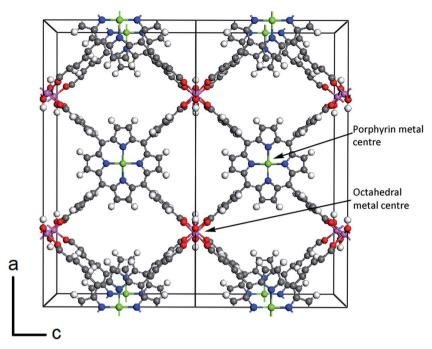
Fig. 1 Perspective view of the conventional unit cell (doubled for clarity) for the porphyrin-based MOF investigated in this study, indicating the positions of the octahedral metal centre and the porphyrin metal centre. Colour code: gray = carbon, white = hydrogen, red = oxygen, blue = nitrogen, magenta = octahedral metal centre, green = porphyrin metal centre. A primitive cell, with half the number of atoms of the orthorhombic cell, was used in our calculations.
