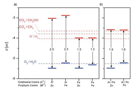
Fig. 4 Band gaps and band edge positions with respect to the vacuum level, as calculated with the screened hybrid functional HSE06 for (a) PMOF with only one element (A = Al or Fe) in the octahedral sites, and (b) mixed PMOF with 50% Al and 50% Fe at the octahedral sites. The energy levels corresponding to redox potentials of water splitting and carbon dioxide reduction reactions producing methane and methanol at pH = 7are also shown with dotted lines
