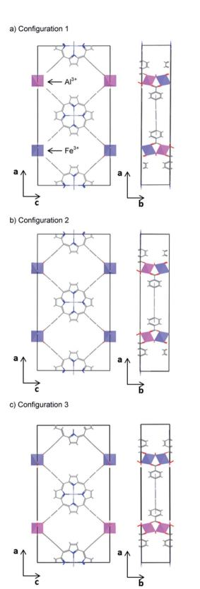
Fig. 5 The three symmetrically independent configurations of Fe and Al on the octahedral sites of the PMOF conventional (orthorhombic) cell.
