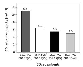
Fig. 7 CO<sub>2</sub> adsorption capacity of APVC/SBA-15 (4%) composites depending on the nature of the aminating reagent.
