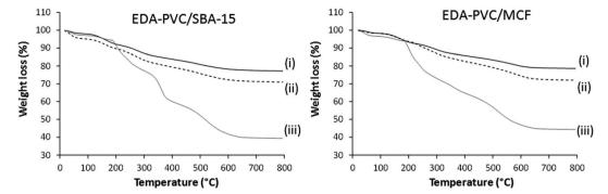
TGA curves for EDA-PVC/SBA-15 and EDA-PVC/MCF samples with (i) 4%, (ii) 7% and (ii) 19% loadings
