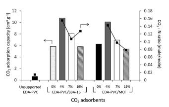
Fig. 6 CO $_2$  adsorption capacity at 25 °C measured by gravimetric method (left scale) and CO $_2$ : N ratio (right scale) for EDA–PVC/mesoporous silica samples depending on the amount of APVC. The CO $_2$ : N ratio is calculated from the CO $_2$  adsorption capacity while the nitrogen content was calculated from CHN analysis.
