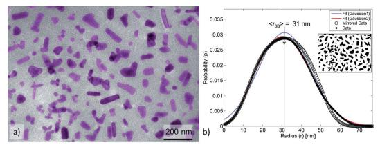
Fig. 3 (a) TEM images of an annealed and densely packed film of ZnO-q-PBMA80k with computer-assisted coloring of ZnO NPs. (b) Fitting of the NP-size by a first and a second order Gaussian distribution and calculation of average radius.
