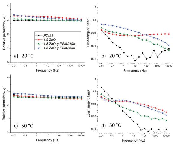
Fig. 11 Dielectric spectroscopy data of neat *PDMS*, 1.5ZnO, 1.5ZnO-g-PBMA10k and 1.5ZnO-g-PBMA60k at 20 °C (a and b) and at 50 °C (c and d). Fig. (a) and (c) show the relative permittivity,  $\varepsilon'_r$  versus frequency, and (b) and (d) the loss tangent,  $\tan \delta$  versus frequency.
