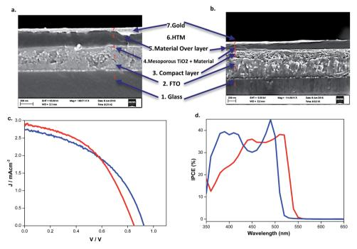
Fig. 9 SEM cross-sectional image of (a)  $(BdA)Pb_2I_6$  and (b)  $(BdA)PbI_4$  based solid-state solar cells showing their related architectures. Obtained (c) current-voltage and (d) IPCE curves of ---  $(BdA)Pb_2I_6$  and ---  $(BdA)PbI_4$  solar cells. A mesoporous  $TiO_2$  layer was used as the electron transporting material and gold was used as the back contact.
