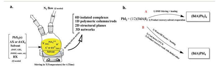
Fig. 1 General solution-based synthetic procedure for organic-inorganic lead halide materials, and (b) the synthetic routes for preparation of the (BdA)Pbl<sub>4</sub> and (BdA)Pb<sub>2</sub>l<sub>6</sub>.
