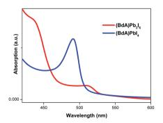
Fig. 4 Absorption spectra of spincoated --- 1D and --- 2D butyl-1,4-diammonium lead( $\shortparallel$ ) iodide materials on TiO<sub>2</sub> films. A small red shift in the band edge is observed for the one-dimensional (BdA)Pb<sub>2</sub>l<sub>6</sub> as compared to two-dimensional (BdA)Pbl<sub>4</sub>, 544 nm and 523 nm, respectively.
