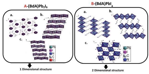
Fig. 2 Crystal structure of (A) solvated (BdA)Pb2l6 and (B) (BdA)Pbl4 (ref. 17) along three axes.
