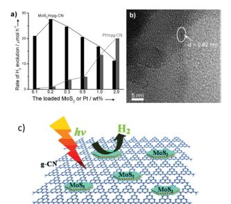
Fig. 6 (a) The rate of  $H_2$  production over mpg- $C_3N_4$  loaded with different amounts of MoS<sub>2</sub> or Pt, (b) TEM image of MoS<sub>2</sub>/g- $C_3N_4$  and (c) illustration of the deposition of layered MoS<sub>2</sub> on the surface of g- $C_3N_4$  for photocatalytic  $H_2$  evolution. Reprinted with permission from ref. 57. Copyright 2013, Wiley-CVH.
