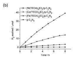
Fig. 8 (a) Structures of Ni-, Co-, and Fe-based cocatalysts and g- $C_3N_4$ , (b) photocatalytic  $H_2$ -evolution for different cocatalyst modified g- $C_3N_4$  samples. Reprinted with permission from ref. 94. Copyright 2012, Wiley-CVH.
