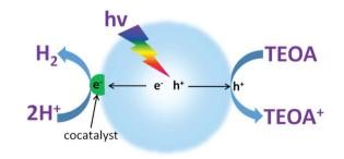
Fig. 3 Schematic illustration of photocatalytic water reduction for  $H_2$  evolution in the presence of an electron donor driven by a semi-conductor modified with  $H_2$  evolution cocatalysts. TEOA: triethanolamine.
