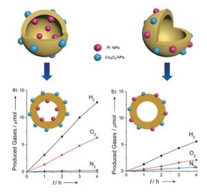
Fig. 13 Time course of the photocatalytic evolution of  $H_2$  and  $O_2$  using (a)  $Co_3O_4/HCNS/Pt$  and (b)  $(Co_3O_4 + Pt)/HCNS$  under UV irradiation ( $\lambda > 300$  nm). Reprinted with permission from ref. 40. Copyright 2016, Wiley-CVH.
