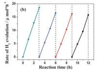
Fig. 7 (a) Comparison of the photocatalytic activity of samples with different amounts of  $Ni(OH)_2$  loaded on  $g-C_3N_4$  polymers, (b) cyclic  $H_2$ -evolution curve for the Ni0.5 sample. Reprinted with permission from ref. 80. Copyright 2013, Royal Society of Chemistry.
