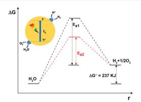
Fig. 2 Schematic description of the energy diagram of a semi-conductor modified with both  $H_2$  and  $O_2$  evolution cocatalysts under light irradiation for non-sacrificial photocatalytic water splitting.  $E_{a1}$ : activation energy without cocatalysts;  $E_{a2}$ : activation energy with cocatalysts;  $\Delta G$ : Gibbs free energy change;  $\Delta G^0$ : Gibbs free energy change under standard conditions; r: redox reaction process.
