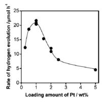
Fig. 4 Dependence of the  $H_2$  evolution rate, when using Pt-loaded g- $C_3N_4$  under visible light, on the loading amount of Pt. Reprinted with permission from ref. 56. Copyright 2009, American Chemical Society.
