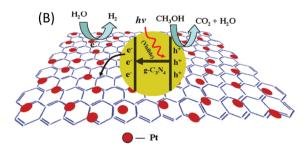
Fig. 9 (A) Comparison of the photocatalytic activities of samples with different loading amounts of graphene on  $g-C_3N_4$  polymers, (B) proposed mechanism for the enhanced electron transfer process of the graphene/ $g-C_3N_4$  polymers. Reprinted with permission from ref. 48. Copyright 2011, American Chemical Society.
