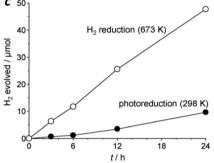
Fig. 5 Size distribution of Pt particles prepared by (a) photoreduction (298 K) and (b)  $\rm H_2$  reduction (673 K); (c)  $\rm H_2$  evolution activities in the presence of an electron donor. Reprinted with permission from ref. 86. Copyright 2014, Royal Society of Chemistry.
