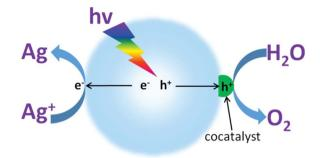
Fig. 10 Schematic illustration of photocatalytic water oxidation for  $O_2$  evolution in the presence of an electron acceptor driven by a semi-conductor modified with  $O_2$  evolution cocatalysts.
