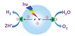
Fig. 1 Schematic illustration of photocatalytic overall water splitting over a semiconductor photocatalyst modified with both  $H_2$ - and  $O_2$ -evolution cocatalysts.
