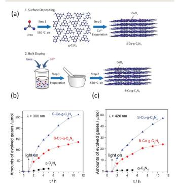
Fig. 11 (a) Schematic illustration of surface modification and bulk doping modification of  $CoO_x$  with  $g-C_3N_4$ . Photocatalytic water oxidation activities of the  $g-C_3N_4$ ,  $B-Co-g-C_3N_4$  and  $S-Co-g-C_3N_4$  samples under (b) UV ( $\lambda$  > 300 nm) and (c) visible light ( $\lambda$  > 420 nm) irradiation. Reprinted with permission from ref. 107. Copyright 2016, American Chemical Society.
