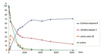
Fig. 1 Monitoring of the hydrogenation of dimethyl 1,6-hexanedioate in the presence of aniline against time. Conditions:  $[Ru(acac)_3]$  (1 mol%), triphos (2 mol%), MSA (1 mol%), dioxane (45 mL), dimethyl 1,6-hexanedioate (1 equiv. 7.5 mmol), aniline (1.5 equiv.), H<sub>2</sub> (10 bar), 220 °C.
