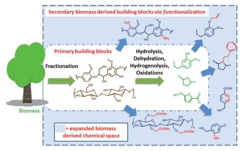
Scheme 1 Schematic representation of the expanded biomass derived chemical space
