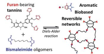
Scheme 15 Thermo-reversible polymer networks prepared from furan-bearing condensed tannins and bismaleimide linkers. Tannin was functionalized through ring-opening reactions with furfuryl glycidyl ether. Reproduced with permission from ref. 100. All rights reserved. Copyright 2017, American Chemical Society.
