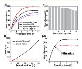
Fig. 6 (a) Reaction kinetic curves of benzene borylation catalyzed by Ir(cod)-homo (black line), Ir(cod)-BPy<sub>0.3</sub>-NT (red line), Ir(cod)-BPy-SBA-15 (blue line), and Ir(cod)-Gbpy-NT (pink line). (b) Reusability of Ir(cod)-BPy<sub>0.3</sub>-NT for benzene borylation. (c) Total TONs of Ir(cod)-BPy<sub>0.3</sub>-NT (black line) and Ir(cod)-homo (red line) for the recycling. (d) Filtration experiment of Ir(cod)-BPy<sub>0.3</sub>-NT catalyst (red-dotted line).
