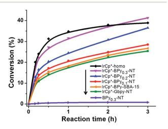
Fig. 4 Reaction kinetic curves of THF oxidation catalyzed by IrCp\*-homo (black line), IrCp\*-BPy<sub>0.3</sub>-NT (pink line), IrCp\*-BPy<sub>0.2</sub>-NT (blue line), IrCp\*-BPy<sub>0.1</sub>-NT (red line), IrCp\*-BPy-SBA-15 (yellow line), IrCp\*-Gbpy-NT (green line), and BPy<sub>0.3</sub>-NT (purple line).
