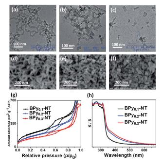
Fig. 1 (a–f) TEM and SEM images of (a and d) BPy $_{0.1}$ -NT, (b and e) BPy $_{0.2}$ -NT, and (c and f) BPy $_{0.3}$ -NT, respectively. Insets in (a–c) are the nanotube length distribution in ethanol obtained *via* dynamics light scattering. (g) Nitrogen adsorption–desorption isotherms and (h) UV/ vis diffuse reflectance spectra of BPy $_{0.1}$ -NT (black line), BPy $_{0.2}$ -NT (blue line), and BPy $_{0.3}$ -NT (red line).
