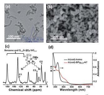
Fig. 3 (a) TEM and (b) SEM images of Ir(cod)-BPy $_{0.3}$ -NT. (c)  $^{13}$ C CP MAS NMR spectrum of Ir(cod)-BPy $_{0.3}$ -NT. (d) UV/vis diffuse reflectance spectra of Ir(cod)-homo (black line) and Ir(cod)-BPy $_{0.3}$ -NT (red line).
