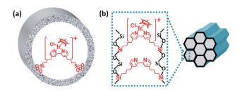
Scheme 4 Schematic of (a) IrCp\*-Gbpy-NT and (b) IrCp\*-BPy-SBA-15.
