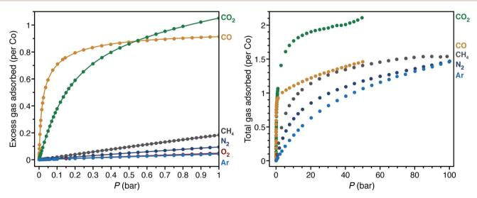
Fig. 4 Low-pressure gas adsorption isotherms for CO (yellow),<sup>40</sup> CO<sub>2</sub> (green),<sup>29</sup> CH<sub>4</sub> (gray), N<sub>2</sub> (dark blue), O<sub>2</sub> (red), and Ar (light blue) at 298 K (left). High-pressure gas adsorption isotherms for CO (yellow), 40 CO<sub>2</sub> (green), CH<sub>4</sub> (gray), N<sub>2</sub>(dark blue), and Ar (light blue) at 298 K (right). The filled circles and solid lines represent experimental data and corresponding Langmuir fits, respectively.
