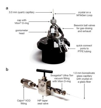
Fig. 2 (a) Diagram of the gas cell, which was designed and built at Advanced Light Source Beamline 11.3.1. (b) Diagram of a capillary-dosing assembly.
