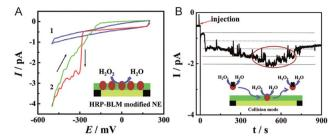
Fig. 5 Studying the single HRP with a BLM-Au nanoelectrode.  $^6$  (A) Cyclic voltammograms of the BLM-Au nanoelectrode (1) and HRP-embedded BLM-Au nanoelectrode (2) in a solution of 20 mM  $\rm H_2O_2$  and PBS buffer (pH: 7.4). (B) Chronoamperometric response of HRP collision into the BLM-Au electrode. Reproduced by permission of ref. 6 from The Royal Society of Chemistry.
