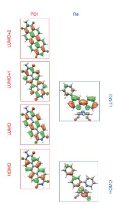
Fig. 7 Frontier molecular orbitals of PDI (left) and  $[Re(Phbpy)(CO)_3-(py)]^+$  molecular fragments calculated using DFT (isovalue = 0.03). Frontier MOs of the full PDI- $[Re(Phbpy)(CO)_3(py)]^+$  dyad are shown in Fig. S15.†
