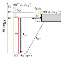
Fig. 9 Jablonski diagram showing electron transfer in PDI<sup>1-</sup>-Phbpy-Re-Py after excitation at 950 nm (red) or 680 nm (yellow). Energy of the charge-transfer state is shown as a range to reflect the uncertainty of the exact energy of this state.
