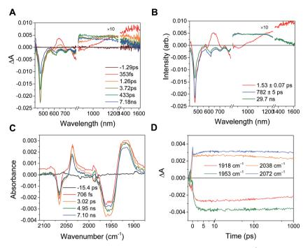
Fig. 10 (A) Transient absorption and (B) species-associated spectra for complex Phbpy-Re-PyPhNDI $^{1-}$  ( $\lambda_{\rm ex}=605$  nm) showing biphasic back electron transfer kinetics. Kinetic traces and fits are shown in Fig. S7.† (C) fsIR spectra and (D) kinetic traces with fits for complex Phbpy-Re-PyPhND1<sup>1-</sup> ( $\lambda_{ex} = 605$  nm) showing monophasic back electron transfer kinetics. The instrument response is approximately 2 ps.
