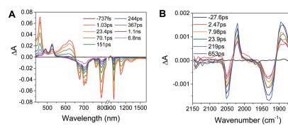
Fig. 3 (A) Transient absorption spectrum of Phbpy-Re-PyPhPDI<sup>1-</sup> ( $\lambda_{ex} = 950$  nm). (B) Time-resolved mid-IR spectrum of Phbpy-Re-PyPhPDI<sup>1-</sup> ( $\lambda_{ex} = 704$  nm).
