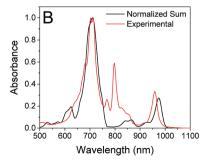
Fig. 8 Left: Calculated vibronic transitions from the ground state to the D1 (black), D2 (red) and D3 (blue) states of PDI<sup>-</sup>. Right: Sum of the three calculated vibronic spectra (black) compared to the experimentally determined spectrum of PDI-, normalized to the maximum value.
