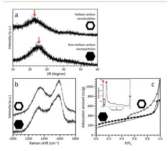
Fig. 3 (a) Wide-angle PXRD patterns, (b) Raman spectra, and (c)  $N_2$  adsorption—desorption isotherms of the non-hollow carbon nanoparticles and hollow carbon nanobubbles. The pore size distribution of the hollow carbon nanobubbles is calculated by the non-local density functional theory (NLDFT) method, as shown in the inset of (c).
