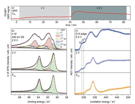
Fig. 1 (a) Oxygen QMS trace, (b) Ir 4f spectra and (c) O K-edges of Ir-coated PEM (120 s Ir sputtered) recorded in the two-electrode cell with the indicated potentials applied (p = 5 Pa, H<sub>2</sub>O).
