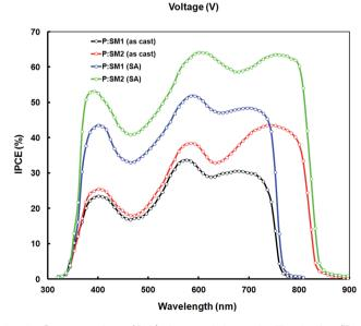
Fig. 5 Current-voltage (J-V) characteristics under illumination (Top) and IPCE spectra of the devices based on P:SM1 and P:SM2 (Bottom).
