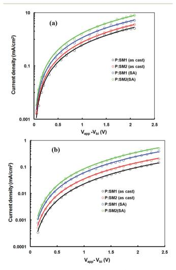
Fig. 6 Current-voltage characteristics in dark (a) hole only devices and (b) electron only devices.
