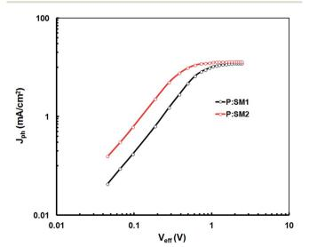
Fig. 7 Variation of  $J_{\rm ph}$  with  $V_{\rm eff}$  for the devices based on P:SM1 and P:SM2 processed with SA (DIO/CF).
