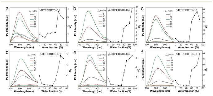
Fig. 1 Study of aggregation-induced emission. PL spectra and plots of the relative PL intensity of  $\alpha$ -DTPEBBTD-Cx and  $\beta$ -DTPEBBTD-Cx in THF/H<sub>2</sub>O mixtures with different volume fractions of water ( $f_w$ ).  $I_0$  and I are the PL intensities of  $\alpha$ -DTPEBBTD-Cx and  $\beta$ -DTPEBBTD-Cx in pure THF ( $f_{\rm w}=0$ ) and THF/water mixtures with specific  $f_{\rm w}$ s, respectively.  $\lambda_{\rm ex}=635$  nm. The concentration is 5  $\mu$ M.
