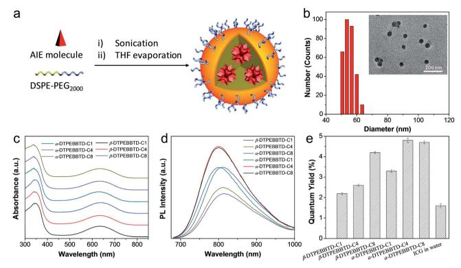
Fig. 2 Preparation and characterization of the AIE NPs. (a) Schematic illustration of AIE NP preparation. (b) Representative LLS and TEM results of  $\alpha$ -DTPEBBTD-C4 based AIE NPs. (c) UV-vis absorption and (d) PL spectra of the AIE NPs in water. (e) Quantum yields of the AIE NPs and ICG in water
