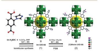
Scheme 1 Syntheses of 1 and 2 via reticular chemistry and by a PSM method, respectively. Green polyhedra: Zr<sub>6</sub> clusters. Yellow ball: micropores. Only part of the linkers are shown for clarity.
