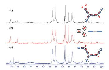
Fig. 3  $^{1}$ H NMR spectra in D<sub>2</sub>O of (a) A<sub>2</sub>–B<sub>3</sub>–CB[8] hyperbranched supramolecular polymer in its equilibrium state; (b) after 1 h of UVA exposure; (c) after subsequent heating at 80  $^{\circ}$ C for 6 h. Note, upon heating the azobenzene is >99% *E* isomer, higher than that originally present in (a).
