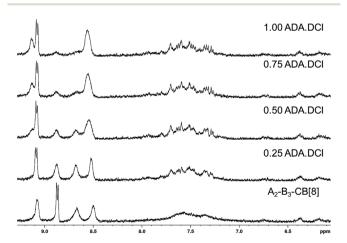
Fig. 4  $^{1}$ H NMR spectra in D<sub>2</sub>O of A<sub>2</sub>–B<sub>3</sub>–CB[8] hyperbranched supramolecular polymer upon titration with up to 1 molar equivalent of ADA·DCl relative to CB[8].
