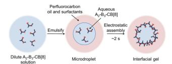
Fig. 5 A schematic outline of the assembly process from dilute solution to an interfacial gel. At dilute solution there are no precipitates as only small polymeric species are present. After emulsification and subsequent electrostatic attraction to the liquid–liquid interface, the concentration and density of the polymer rapidly increases over *ca.* 2 s, leading to inter-polymeric crosslinking and gelation to occur (Fig. 6b).
