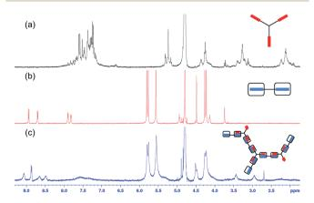
Fig. 2  $\,^{1}$ H NMR spectra in D<sub>2</sub>O of (a) B<sub>3</sub>, (b) A<sub>2</sub>-CB[8] (1 : 2), (c) A<sub>2</sub>-B<sub>3</sub>-CB[8] (1.5 : 1 : 3) SHP. Concentrations in all cases were A<sub>2</sub> = 0.55 mM, B<sub>3</sub> = 0.37 mM, CB[8] = 1.11 mM.
