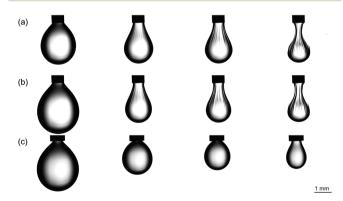
Fig. 8 Transmission optical micrographs of the pendant droplet during IFT measurements of continuous aqueous A2-B3-CB[8], and droplet of 0.001 wt% K<sup>-</sup> in FC-40. From left to right, (a) equilibrated 5 μL droplet pumped in and exhibiting a buckled phase change; (b) droplet after subsequent pumping out to 8.5 µL followed by immediate pumping in; (c) droplet containing 0.01 wt% K<sup>+</sup> in FC-40 and subsequent pumping in.
