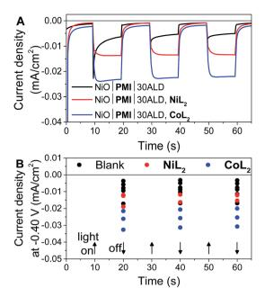
Fig. 6 (A) Current density measurements with three 10 s light on/off cycles with -0.40 V applied bias on a single NiO|PMI|30ALD working electrode without catalyst (black, "blank") and again after additional 0.5 mM NiL2 (red) or 0.5 mM CoL2 (blue). (B) Results of the same experiment with  $5\!-\!30$  cycles of Al2O3 ALD from Fig. S16.† The number of cycles of ALD is not distinguished for clarity (conditions: 0.1 M  $_{2}$ O4 and 0.1 M  $_{2}$ O4 in 1:1  $_{2}$ O: MeCN).
