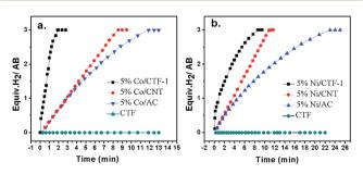
Fig. 3 Plots of volume of  $H_2$  generated vs. time for AB hydrolysis catalyzed by (a) 5% Co/CTF-1, 5% Co/CNT, 5% Co/AC, CTF (b) 5% Ni/CTF-1, 5% Ni/CNT, 5% Ni/AC, CTF. ([AB] = 322 mM, 5 mL,  $n_{\rm metal}/n_{\rm AB}$  = 0.05).
