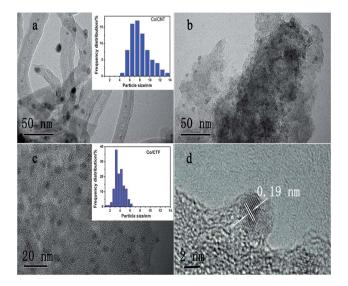
Fig. 2 TEM images and corresponding size histograms of (a) 5% Co/ CNT, (b) 5% Co/AC, (c) 5% Co/CTF-1, (d) high resolution image of Co particles on CTF-1. The average size is calculated from at least 100 nanoparticles
