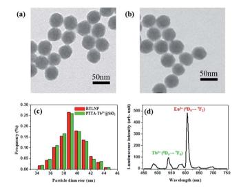
Fig. 3 TEM images of PTTA-Tb<sup>3+</sup>-encapsulated silica particles (a) and RTLNP particles (b). (c) Particle size distribution histograms of the two kinds of nanoparticles. (d) Time-gated emission spectrum of the RTLNP (50  $\mu g$  ml $^{-1}$ ) in 1 : 4 ethanol-0.05 M PBS buffer of pH 7.4 ( $\lambda_{ex}$  = 330 nm).
