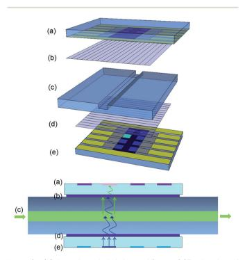
Fig. 3 (top) Schematic exploded view and (bottom) 2D edge view of OLEC excitation and OPD detection system with a glass microfluidic device and polarization filters: (a) fully solution processed OPD; (b) first linear polarization filter oriented at 0 degree; (c) glass microfluidic chip; (d) second linear polarization filter oriented at 90 degree; (e) fully solution processed blue OLEC.
