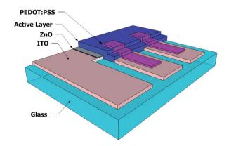
Fig. 1 Layer architecture diagram (quarter part of full device) of fully solution processed blue OLEC and OPD on ITO glass substrate. Both OLEC and OPD share exactly the same inverted layer structures: ITO (100 nm)||ZnO (20 nm)||active layer (200 nm)||PEDOT:PSS (40 nm). For blue OLEC, the active layer consists of blue light-emitting polymer SPB-02T, solid electrolyte DCH18C6 and dopant LiTf with a mass ratio of 1:1:0.27. For OPD, the active layer consists of P3HT: PCBM with 1:1 mass ratio.
