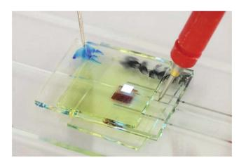
Fig. 2 OLEC excitation and OPD detection system with a glass microfluidic device. For illustration reasons, the linear polarization filters are not integrated. The blue illuminating square is the illuminating blue OLEC pixel; the dark reds square is the active layer of OPD; the glass channel is in-between the OLEC and the OPD.
