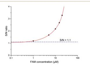
Fig. 9 S/N ratio as a function of concentration of FAM dye as OLEC driven at 20 V pulses. Solid red line predicted trends for the theoretical LOD at S/N = 1.1, which is shown with a dashed blue line.
