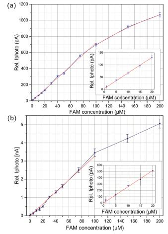
Fig. 8 Fluorescent detection measurement by integrated OLEC and OPD with different FAM dye concentration in water. The FAM solution was excited by the blue OLEC with brightness of (a)  $500 \text{ cd m}^{-2}$  and (b)  $2000 \text{ cd m}^{-2}$ ; the inset graph is the zoom-in of the low concentration part (1 to  $20 \mu \text{M}$ ).
