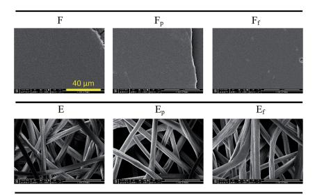
Fig. 2 Topography of PS substrates with varied treatments. A positive control substrate (cellulose filter paper) is added. All images are shown at the same magnification.
