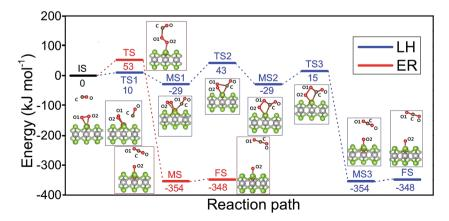
Fig. 6 Configurations of IS, TS, MS and FS along the MEP of CO oxidation catalyzed by  $Fe-PtSe_2$  via the LH (blue) and ER (red) mechanisms, with the corresponding energy profiles. The end points (FS) of LH and ER mechanisms are the same (physisorbed  $CO_2$ ).
