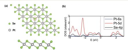
Fig. 1 (a) Top and side views of a  $4 \times 4$  UC of PtSe<sub>2</sub>. The position of Se atom to be replaced with the TM (TM = Sc–Zn) atom is denoted with a red circle. (b) The LDOS projected on the Pt(5d), Pt(6s) and Se(4p) orbitals. The brown dash line indicates the Fermi level (eV).
