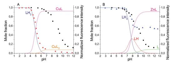
Fig. 3 Fluorescence emission pH titration curves of compound 5 (10  $\mu$ M,  $\lambda_{ex} = 472$  nm,  $\lambda_{em} = 552$  nm) in water in the absence (black  $\blacksquare$ ) or presence of 1 equivalent of metal ion, (A) Cu(II) (red  $\blacksquare$ ) and (B) Zn(II) (blue  $\blacktriangle$ ), and mole fraction distribution diagrams for the various species of this ligand under these conditions (solid lines).
