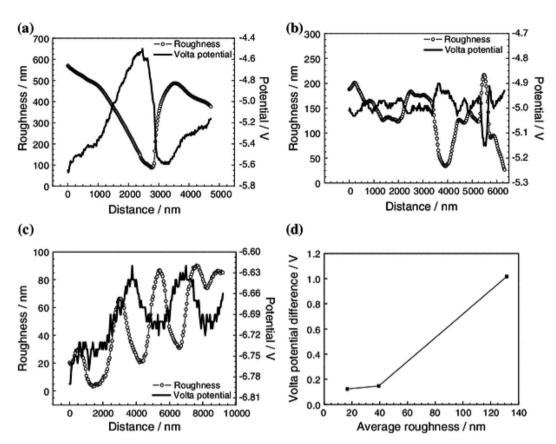
Fig. 17 Image shows line diagram (cross sectional) between roughness and Volta potential with average roughness of (a) Ra 108.0 nm, (b) Ra 39.3 nm, (c) Ra 16.7 nm. (d) Shows Volta potential difference between peak and valley with respective average roughness. Perinted from ref. 152 with permission of Springer. Springer Science + Business Media Dordrecht 2013.
