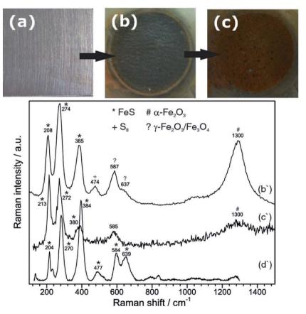
Fig. 14 Shows images of (a) bare metal before exposure to saline  $H_2S$  saturated acetic solution, (b) area of exposure after anodic polarization for 44 h at 200 mV above  $E_{corr.}$  with Raman spectrum (b'); and (c) corrosion products after aging in air for 90 d, with Raman spectrum (c'), along with the reference Raman spectrum for mackinawite (d'). <sup>125</sup> Reproduced by permission of The Electrochemical Society.
