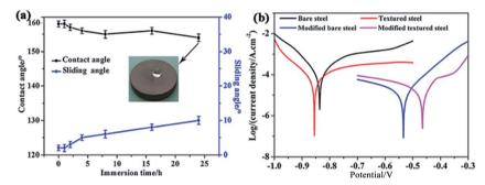
Fig. 6 (a) Establishing relationship between the contact angle and sliding angle of the superhydrophobic surface with the immersion time (3.5% NaCl solution); (b) exhibited the effect of surface modification on polarization behaviour as polarization curves for the bare steel, the textured steel, the modified bare steel, and the modified textured steel are found different.<sup>49</sup> Reprinted with permission from ref. 49. Copyright 2015, Elsevier B. V.
