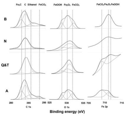
Fig. 12 Presence of C, O and Fe has been confirmed due to the appearance of C 1s, O 1s and Fe 2p regions in XPS high resolution spectra recorded from corroded steel surfaces with different microstructures. Per Reprinted with permission from ref. 100. Copyright 2015, Elsevier B. V.
