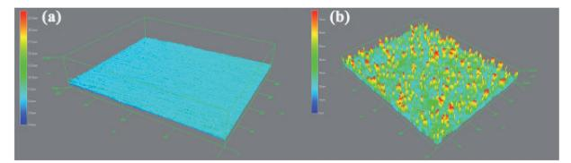
Fig. 5 Surface profile variations in (a) the bare steel and (b) the textured steel surface.<sup>49</sup> Reprinted with permission from ref. 49. Copyright 2015, Fisevier B. V.
