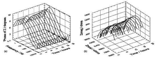
Fig. 11 In situ (a) EIS Bode phase angle and (b) complex-plane impedance plots data for a polished mild steel electrode immersed in 3% (w/v) NaCl saturated with high purity carbon dioxide at atmospheric pressure (adjusted to pH 4.75).<sup>90</sup> Reprinted with permission from ref. 90. Copyright 2007, Elsevier B. V.
