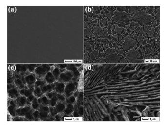
Fig. 4 Morphological images recorded via SEM clearly elucidate the differences for (a) the bare steel and (b) the textured steel surface. (c and d) Magnified images of (b).49 Reprinted with permission from ref. 49. Copyright 2015, Elsevier B. V.
