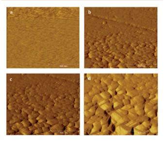
Fig. 7 In situ AFM topographical images of (a) untreated (bare) carbon steel before immersion, and in brine containing DPC (500 ppm) after (b) 5 min, (c) 30 min, and (d) 4 h immersion.83 Reprinted with permission from ref. 83. Copyright 2014, American Chemical Society.
