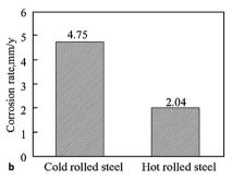
Fig. 1 (a) Comparison of the corrosion rates of cold and hot rolled steel by weight loss (WL), potentiodynamic polarization (PD) and electrochemical impedance spectroscopy (EIS) measurements; (b) comparison of weight loss measurements for cold and hot rolled steel after 6 h immersion in 16.9 vol% H<sub>2</sub>SO<sub>4</sub> and 0.35 vol% HCl solution at 60 °C (pH-0.3).<sup>29</sup> Reprinted from ref. 29 with permission of Springer. Pleiades Publishing, Ltd., 2014.
