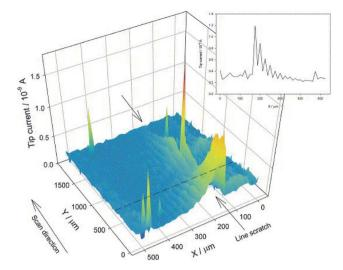
Fig. 19 SECM image of tinplate with a line scratch immersed in 10 mM  $H_2SO_4$ . The current increase above the scratch shows the oxidation of  $Fe^{2+}$  to  $Fe^{3+}$ .  $E_{tip}=+600$  mV,  $E_{sample}=OCP$  (about 520 mV), SECM Pt tip radius: 10  $\mu$ m.<sup>168</sup> Reprinted with permission from ref. 168. Copyright 2006. Elsevier B. V.
