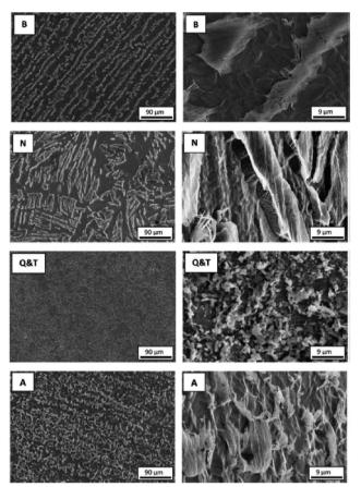
Fig. 13 Appearance of morphological differences after corrosion (with hold time of 6 h in 0.5 M NaCl solution saturated with  $CO_2$ ) of banded (B), normalized (N), quenched and tempered (Q & T) and annealed (A) steels shown by SEM morphological images with two different magnifications. <sup>100</sup> Reprinted with permission from ref. 100. Copyright 2015, Elsevier B. V.
