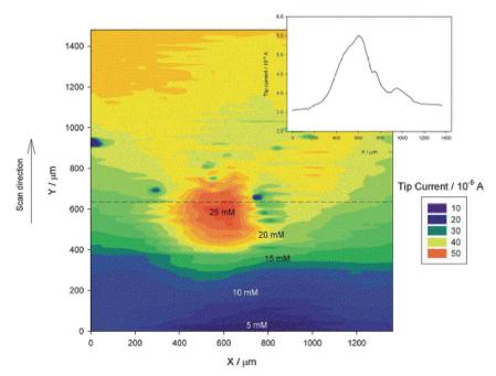
Fig. 20 SECM contour plot exhibiting defect in tin plate which was immersed in 10 mM  $H_2SO_4$ .  $E_{tip} = +600$  mV,  $E_{sample} = OCP$  (about 520 mV), SECM Pt tip radius = 10  $\mu$ m. <sup>168</sup> Reprinted with permission from ref. 168. Copyright 2006, Elsevier B. V.
