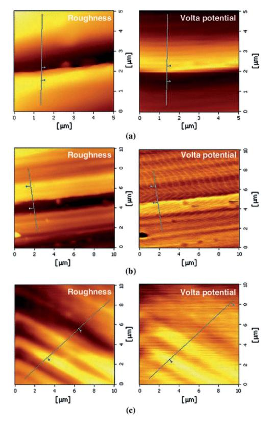
Fig. 16 KPFM image representing topography and Volta potential with different average roughness; (a) Ra 108.0 nm, (b) Ra 39.3 nm, and (c) Ra 16.7 nm. Exprinted from ref. 152 with permission of Springer Science + Business Media Dordrecht 2013.
