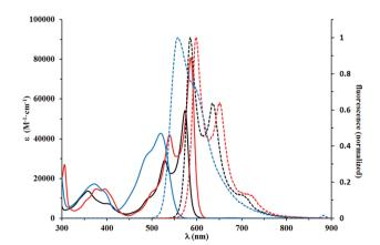
Fig. 3 Absorption (solid lines) and normalized emission (dashed lines) spectra of 5d (black)and 5e (red), which have electron-donating substituents on the benzofuran ring, and 5l (blue), which was modified with only one OMe group. Spectra were measured in DCM.
