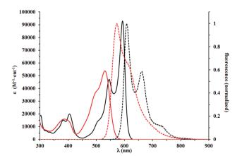
Fig. 2 Absorption (solid lines) and normalized emission (dashed lines) spectra of 5j (black) and 5k (red). All spectra were measured in DCM. Compound 5k was characterized by a lower degree of conjugation between the benzofuran moiety and the DPP core.
