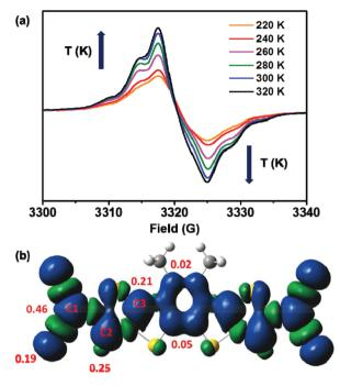
Fig. 3 (a) Variable-temperature EPR spectra of 4CN-DTmBDT in the solid state. (b) Spin-density of the triplet state of 4CN-DTmBDT calculated with DFT using the U3BLY/6-31G(d) level of theory.
