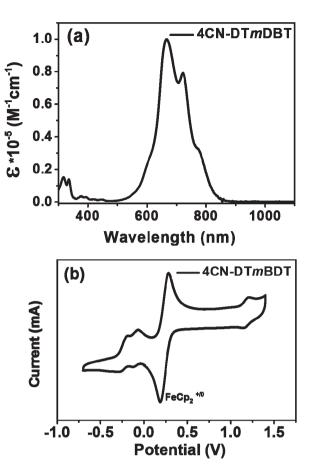
Fig. 4 (a) UV-vis absorption spectrum of 4CN-DTmBDT in  $CH_2Cl_2$  and (b) the cyclic voltammogram of 4CN-DTmBDT in  $CH_2Cl_2$  with  $Bu_4NPF_6$  as the supporting electrolyte, at a scan rate of 100 mV s<sup>-1</sup>.
