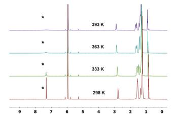
Fig. 2 Variable-temperature  $^1\text{H}$  NMR spectra of 4CN-DTmBDT in  $C_2D_2Cl_4.$
