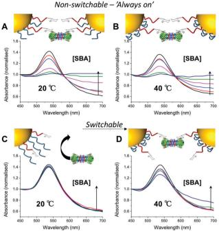
Fig. 2 UV-Vis traces of different nanoparticle formulations in presence of serial dilution of SBA (10-1  $\mu$ g mL<sup>-1</sup>) after 30 minutes incubation. All particles (60 nm) had [pHEA<sub>15</sub>-Gal]: [pNIPAM<sub>x</sub>] 8:2. pNIPAM<sub>25</sub> at 20 °C (A) and 40 °C (B); pNIPAM<sub>50</sub> at 20 °C (C) and 40 °C (D). An increase in  $Abs_{700}$ and decrease in Abs<sub>540</sub> is indicative of binding. All curves normalise so  $Abs_{450} = 1.$
