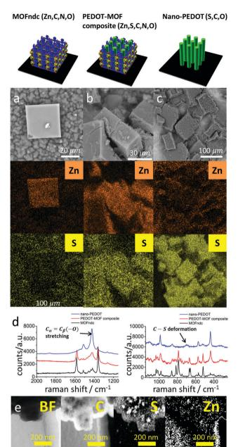
Fig. 2 BSE-SEM images with EDS mappings of Zn and S for (a) MOFndc, (b) PEDOT-MOF composite and (c) nano-PEDOT. Raman spectra (d) extended scan (left) and static scan (right) around 700 cm<sup>-1</sup> Raman shift. (e) Energy filtered transmission electron microscopy (EFTEM) images with EELS mappings of C (K-edge, 284 eV), S (L-edge, 165 eV) and Zn (L-edge, 1020 eV).
