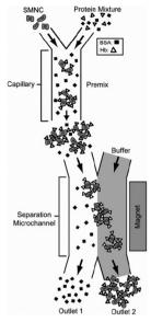
Fig. 4 Superparamagnetic magnetite nanocrystal clusters (SMNC) selectively attach to the hemoglobin, and the conjugated hemoglobin particles are separated from the mixture of unbound bovine serum albumin when the magnetic field is introduced to the channels. Reproduced from ref. 88 with permission from SpringerLink.
