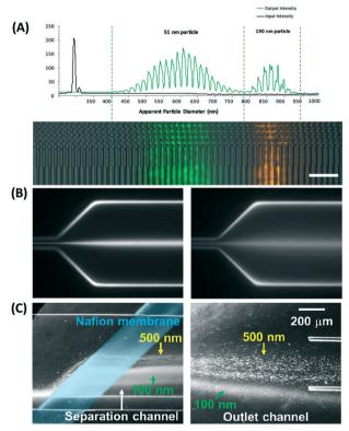
Fig. 14 Wider separation spread caused by Brownian motion of nanoparticles in (A) electrostatic DLD of 50 nm and 190 nm nanoparticle size. Reproduced from ref. 53 with permission from The Royal Society of Chemistry (B) 500 and 200 nm in viscoelastic flow separation. Reproduced from ref. 145 with permission from The Royal Society of Chemistry, and (C) 100 nm nanoparticle size with ion concentration polarization. Reproduced from ref. 137 with permission from Nature Publishing Group.
