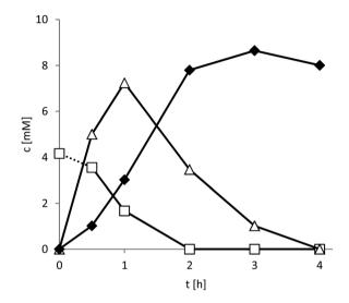
Fig. 3 Time course of the photoenzymatic oxidation of meso-3methyl-1,5-pentanediol ( $\square$ ) to (S)-4-methyltetrahydro-2H-pyran-2-one (♠) via the intermediate lactol (△). General conditions: 100 mM glycine-NaOH buffer (pH 9), 100 mM.  $[diol]_0 = 10$  mM,  $[NADH]_0 = 1$  mM, [FMN] = 100  $\mu$ M, [HLADH] = 7.4  $\mu$ M, 5 drops of catalase, T = 30 °C.
