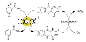
Scheme 1 Aerobic oxidation of reduced nicotinamide cofactors (NAD (P)H) to the corresponding cofactors (NAD(P)+) using photoexcited flavin catalysts. Upon photoexcitation ( $\lambda = 450$  nm) the redox potential of the oxidised flavin catalyst increases dramatically 16 enabling fast hydride transfer from NAD(P)H to the flavin. The reduced flavin reacts spontaneously in a dark reaction with molecular oxygen.<sup>14</sup>
